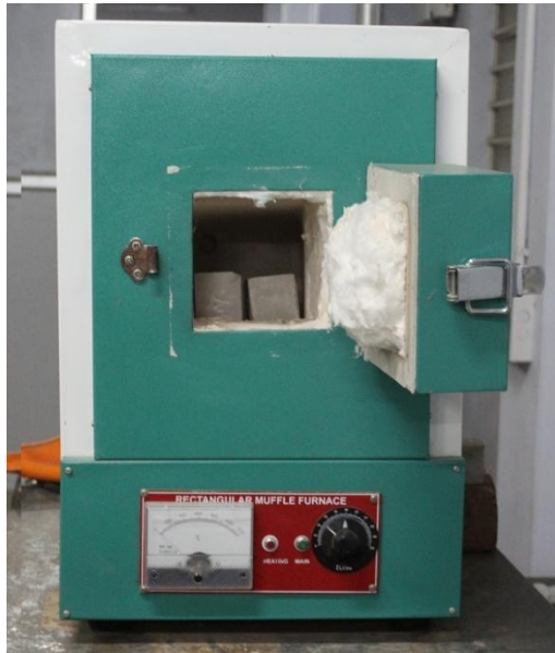
Figure 1 Test setup for elevated temperature attack
